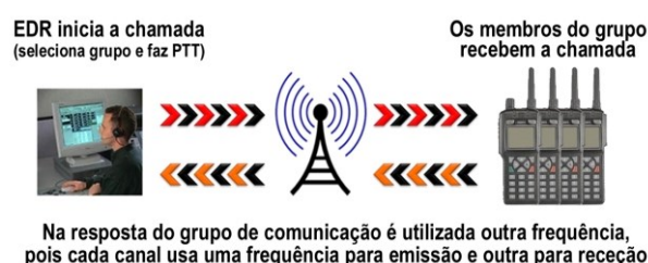
Fig. 49 - TMO - Trunked Mode Operation (Semi-duplex)
